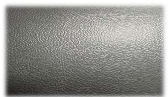
Double sided embossed galvanized products
