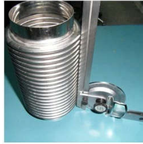
Bellows Verticality Inspection
