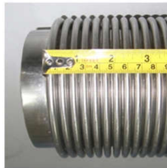
Bellows Shaping Inspection
