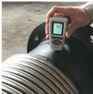
Paint Thickness Inspection
