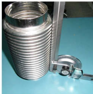
Bellows Verticality Inspection
